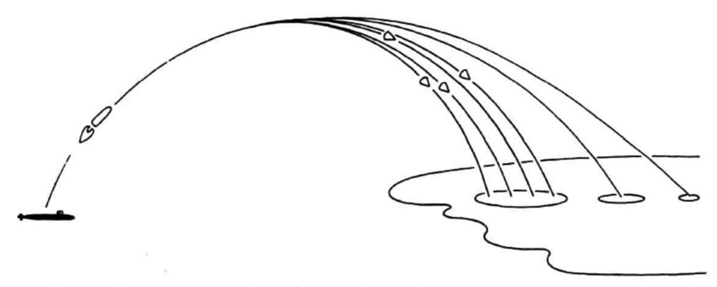
Note: If some of the propulsive energy in the bus is first used to extend the range at which warheads are delivered, there will be less energy available to disperse warheads at a later time. The size of the footprint at extended ranges will therefore be smaller.
