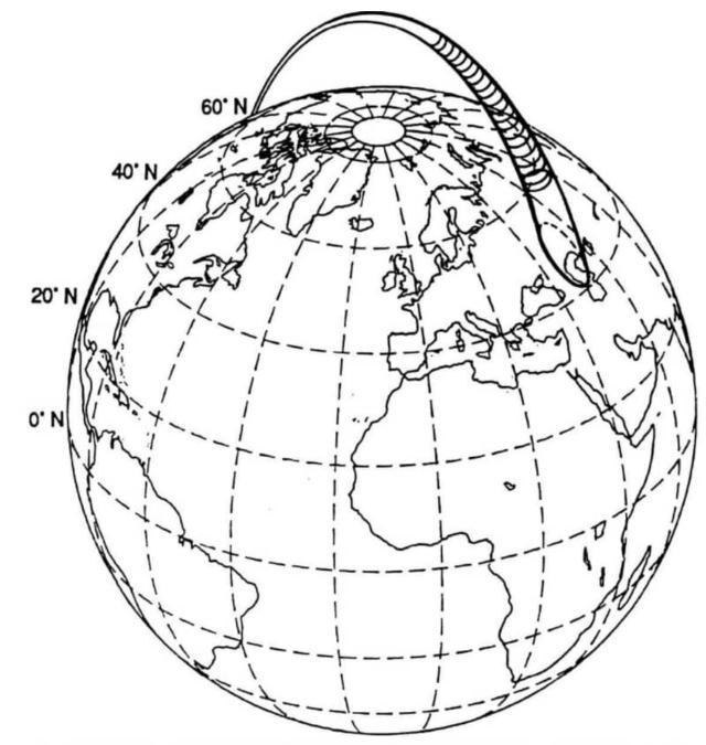
Note: The footprint of a missile is the area within which a MIRVed missile can disperse warheads. It is determined in part by the amount of velocity imparted to each warhead by the post-boost vehicle ("bus"). The finite propulsive energy of the bus and the trajectory' on which the booster launches it also affect the size and shape of the footprint.
